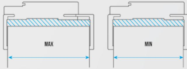
RESİM 4: PERVAZ ÇALIŞMA PAYLARI / PICTURE 4: FRAME WORKING MARGINS
